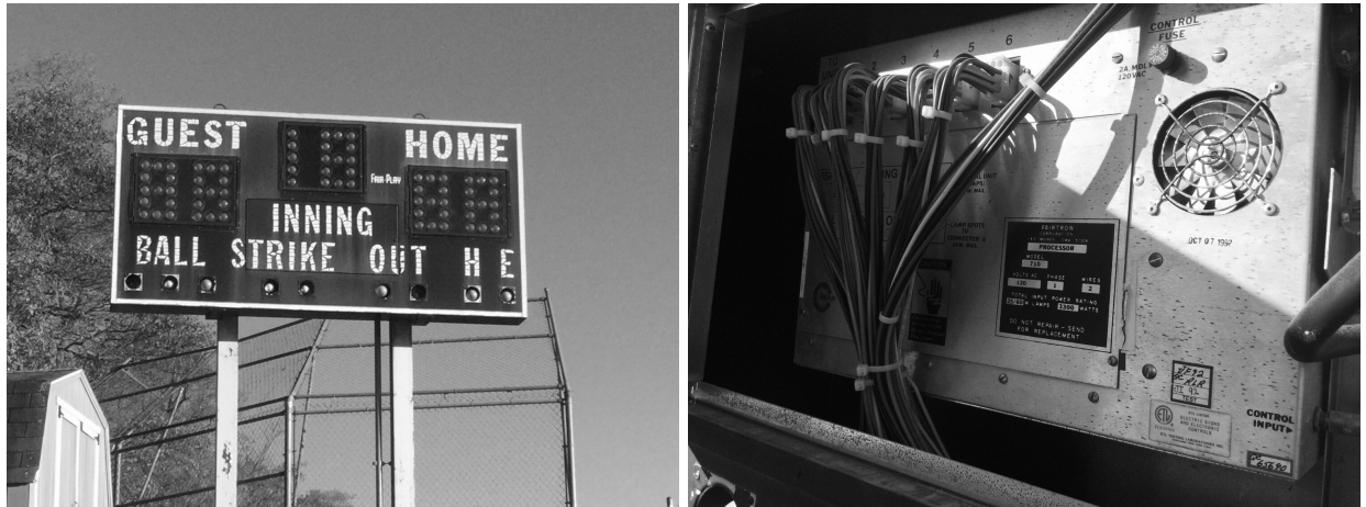
Figure 2: FairPlay 710 scoreboard and internal processor box.
