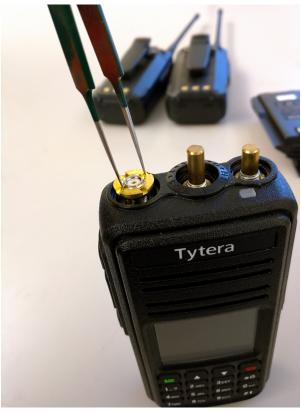
To open your radio, first remove the battery and the four Torx screws that are visible from the back of the device. Then unscrew the antenna and carefully pry off the two knob covers. Beneath each knob and the antenna, there are rings that screw in place to secure them against the radio case; these should be moved by turning them counter-clockwise using a pair of sturdy, dull tweezers.
