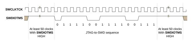
Figure 12 – JTAG-to-SWD sequence timing
